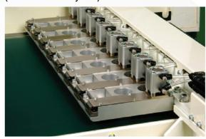
Multiple panels can be held at once by the multiple chucks. Max. 607 mm width.
